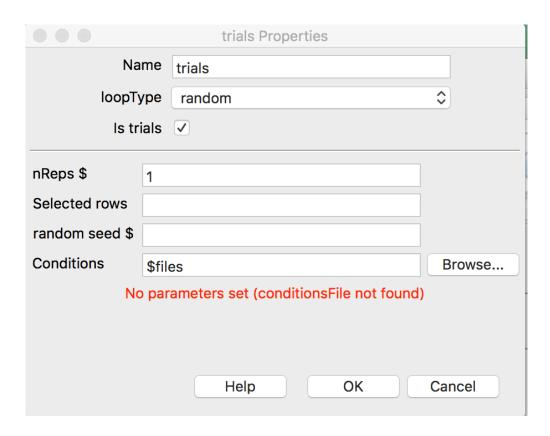
In the trials loop, instead of reading in an Excel sheet for our conditions, we use the column name that lists the files in *SblockOrder.xlsx*. This ensures that a random file is selected each time and used to present only those trials. Below is what one of these files looks like:
